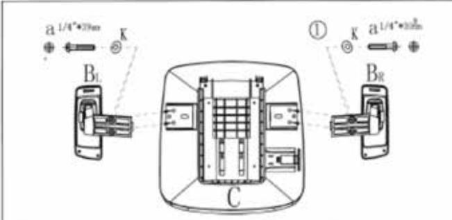
Diagram 1: Attaching armrests  $B_L$  and  $B_R$  to the seat mechanism  $C$  using screws  $a$  ( $1/4 \times 20mm$ ).
