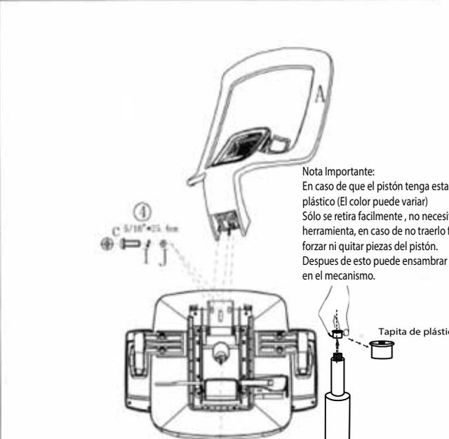
Diagram 2: Attaching the backrest  $A$  to the seat mechanism  $C$  using screw  $j$  ( $5/16 \times 25$  mm). Includes a note about the plastic cap and the piston.
